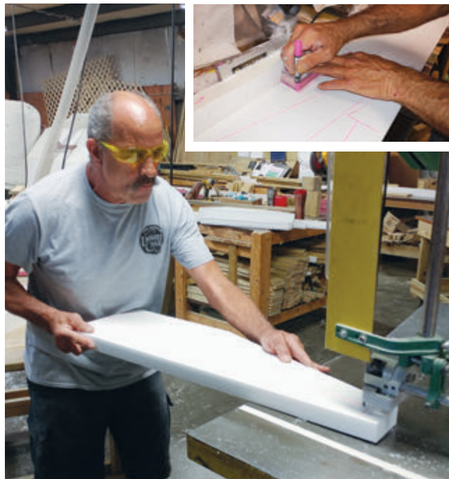
Top: Patterns for chair parts hang on the wall. Center: Jasper Chavis uses the patterns to trace lines on the boards; then he cuts out the chair parts with a bandsaw. Bottom left: Brittany Sechrist assembles a bench.
